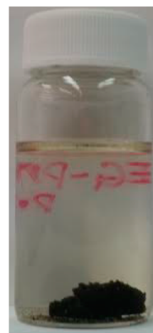
Figure 11. Result of the extraction of oil from oil sands using 60 mg of dodecane instead of toluene. T_{ex} = 50 °C.
